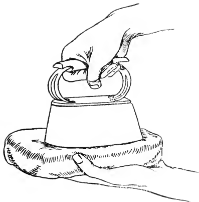
A HOT IRON MELTS THE FINISHERS' GREASE INTO THE LURE
